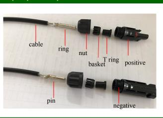
Step 4: cut the cable before installing the connector (strip 9mm).
