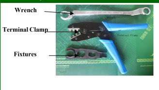
Step 2: (1) Adjustment of riveting pressure: loosen the screw on the pressure ring with a crosshead screwdriver and rotate the adjusting plate (counterclockwise rotation can increase the pressure, otherwise the pressure will decrease). See picture A.
