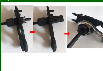
Step 10: adjust the clearance of the nut to 0.2 - 0.8 mm.
